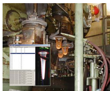
Measurement of molten glass drops size
