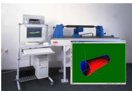
Measurement of rubber printing rollers dimensions
